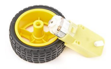
Description: Voltage: DC3-6V Reduction ratio: 1:48 Torque: 0.8kg.cm Tire diameter: 65mm Tire thickness: 28mm
